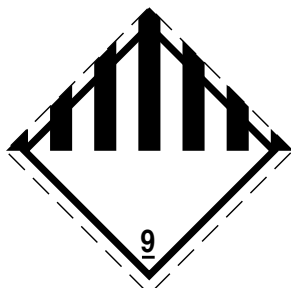
Figure 7.21 CDG hazard placard
