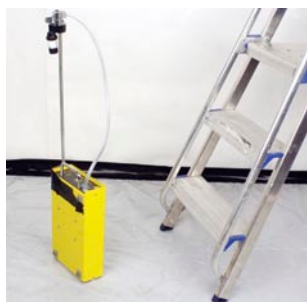
Figure 7.27 Air sampling during clearance
